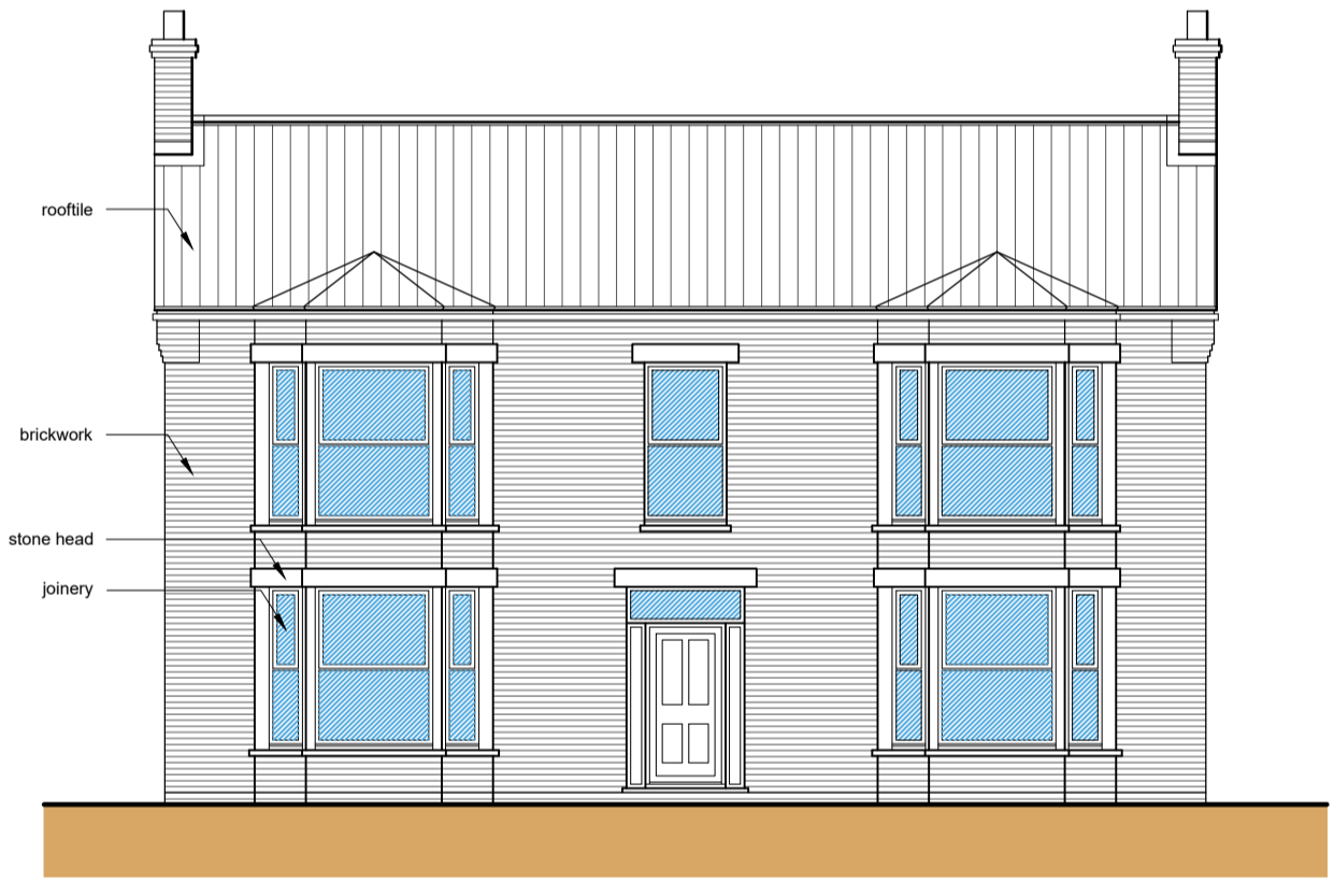
Front Elevation (NW) Scale 1:100 metres
